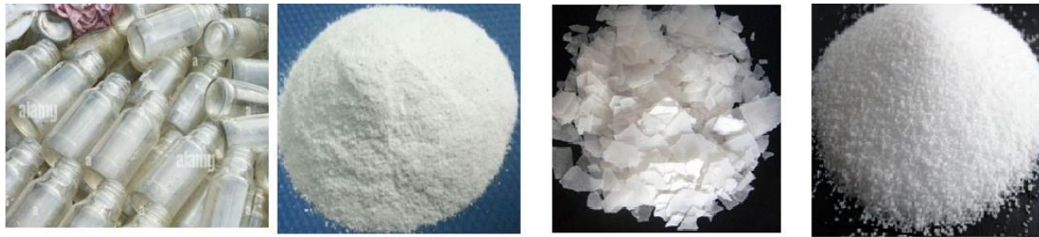
Fig.1. (e) - scrap glass (f) -processed Scarp glass (g)- NaOH (h)- Na 2 SiO 3
