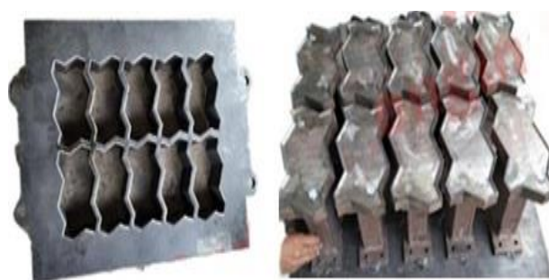
Fig. 2. (a). Mould (b) Casting of block
