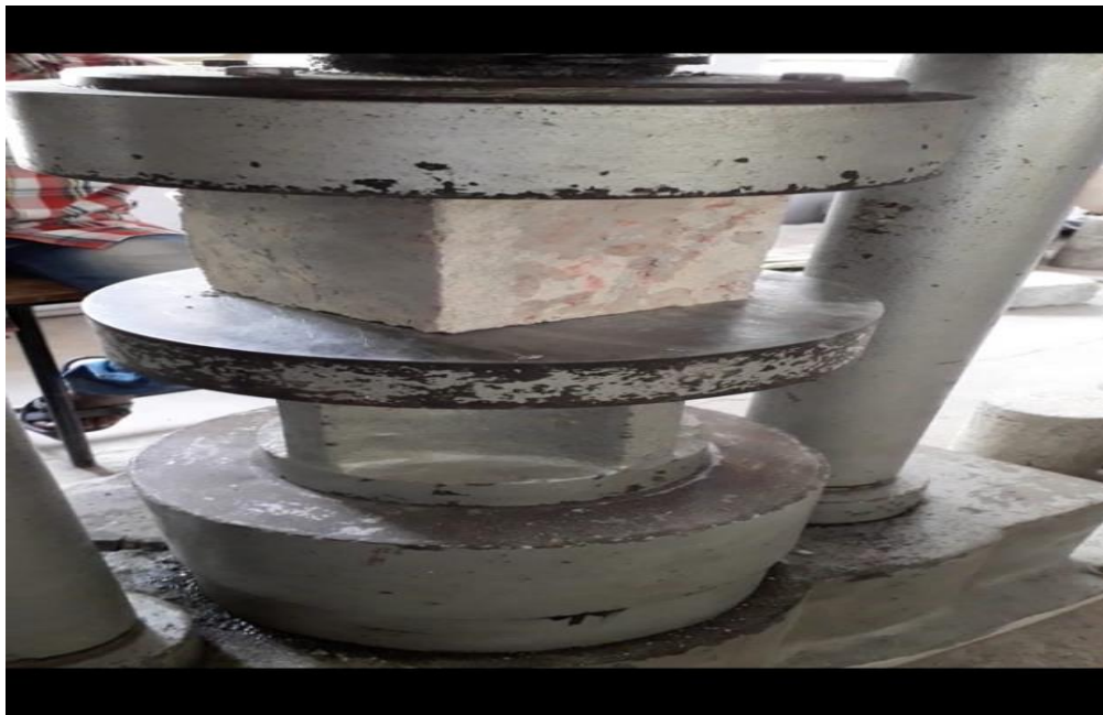
Fig. 2: Compressive strength testing set up
