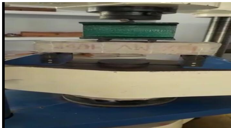
Fig. 4: Flexural strength testing set up
