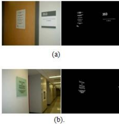
Fig. 4. Indoor nameplate images with different font sizes, perspective distortion, colors and strong reflections (a) Original images (b) Extracted text
